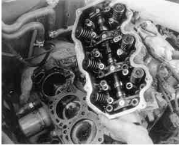
Fig. 23: The cylinder head gasket must be replaced upon installation — VG30E engine
